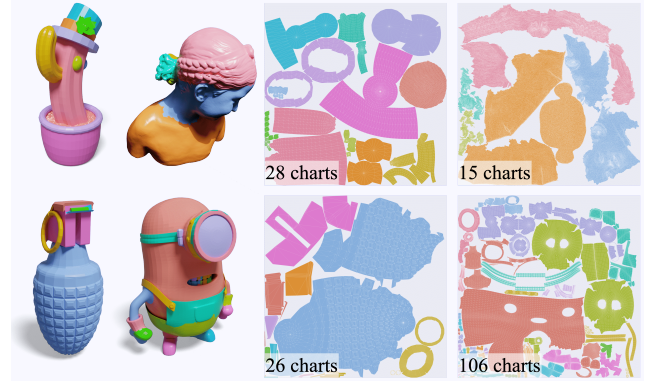
Figure 4: Mesh parameterization maps a 3D surface to a 2D domain (UV space) by partitioning it into charts and flattening each into a planar region. Example meshes (left) and UV layouts (right) show varying chart counts. Figure adapted from [WWS*25].
